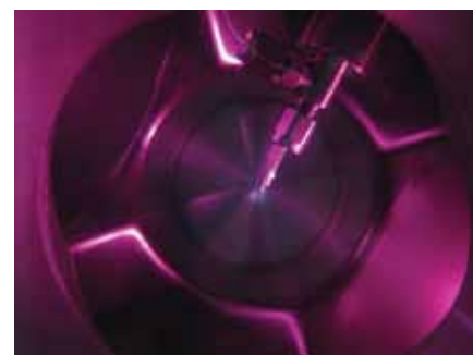
The attosecond pulse source. An intense laser comes in from the left and creates a plasma in the vacuum chamber (purple glow at centre). The excited plasma emits extreme ultraviolet light in a single burst with attosecond pulse duration.
