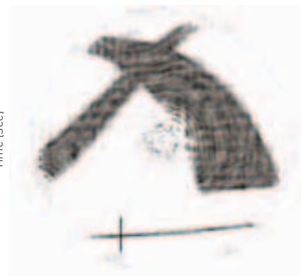
Reconstruction of an Xradia "X" pattern from X-ray data measured using FRIEND.
