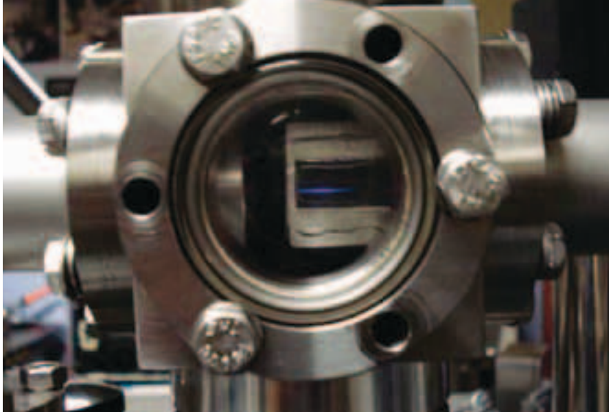
Figure 8: Semi-infinite gas cell for generation of high order harmonics.
