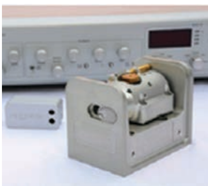
Prototype cat-eye laser (see DJ Thompson and RE Scholten, Narrow linewidth tunable ECDL using wide bandwidth filter Review of Scientific Instruments 83 023107, 2012).
