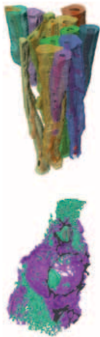
Figure Z: 3D phase retrieval images after segmentation step for 200µm aerosil grain (upper) and 300µm cylindrical structure of secondary osteon in human cortical bone (lower).
