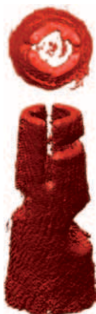
Figure C: The first Fresnel coherent X-ray tomographic reconstruction of a test object in the soft X-ray regime (Isaac Peterson, unpublished). The diameter of the object is 4 \mu\text{m} at its base. Data were collected with FRIEND at the Advanced Photon Source.
